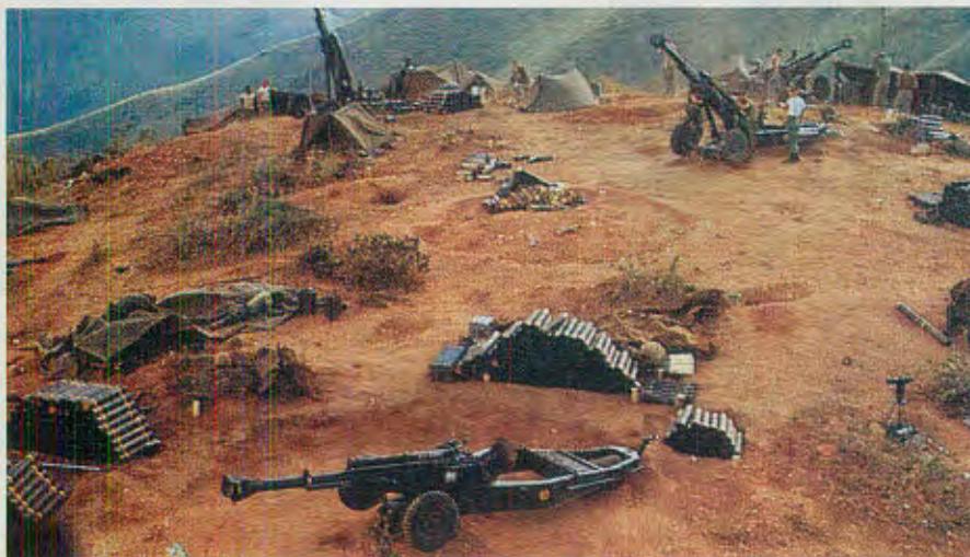
Army firebase in the highlands: Well-sited artillery from these M102 105mm howitzers could provide fire support to a radius of 15 clicks with RAP ammo. We fired more arty, dropped more bombs in Vietnam than in all of WW II... but it didn't work.
